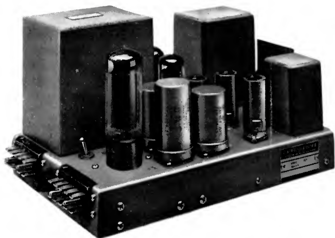
Rear view of BA-14-A Amplifier, showing plug-in construction.
